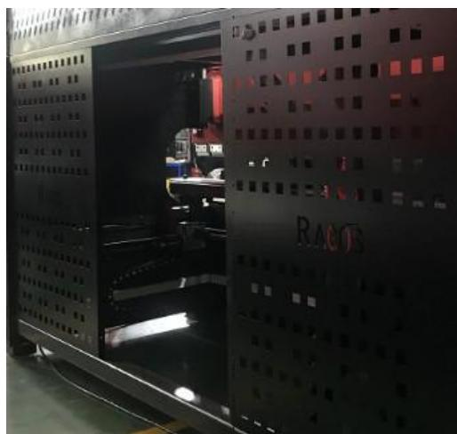
Safety door at the back, the machine will stop and power cut off when the door is accidentally opened to prevent safety accidents caused by the back-gauge movement.
