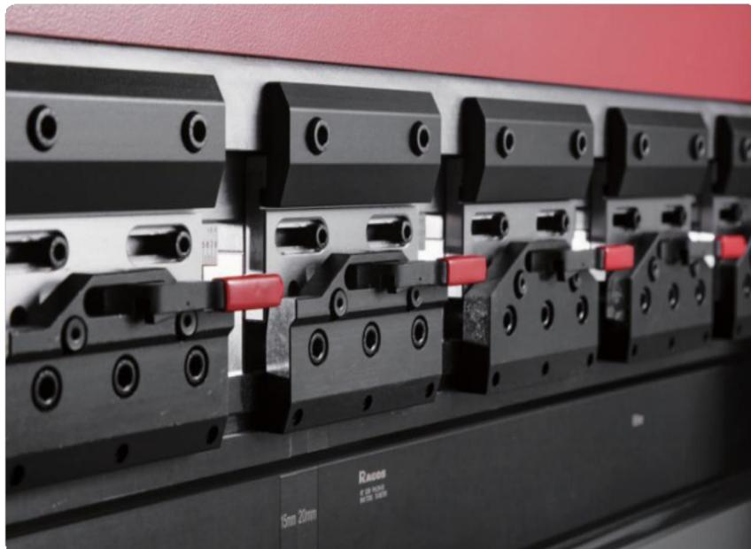
(2) Segmented upper moulds of varying lengths are available and can be assembled to a certain width according to the requirements of the workpiece to suit the processing needs of special workpieces.
