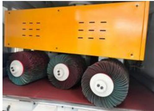
**Universal Roller Brush:** By alternately rotating and spinning the roller brush, the sand belt roller brush can grind the workpiece without dead corners, thereby achieving deburring and fillet machining
