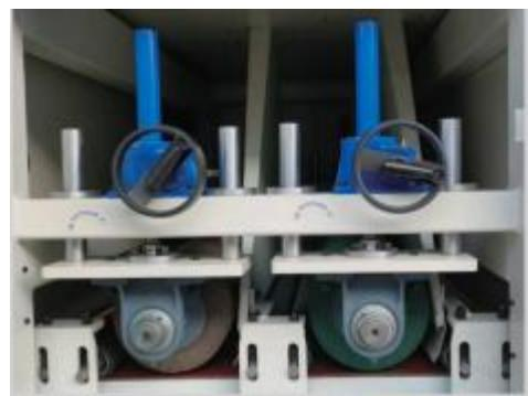
**Polishing Rollers :** Polishing rollers are used for rough grinding or all metal, plastic and other workpieces removing metal burrs, sanding, drawing, grinding decorative patterns, grinding, matte, soft light.etc They are mainly used for grinding stainless steel special fine sand patterns, polishing and mirror treatment.
