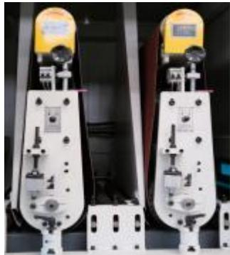
**Double sand belts:** The equipment is equipped with two sets of wide sanding belt mechanisms, which rotate at high speed to remove burrs, oxide scales, polishing,etc. on the surface of the workpiece.
